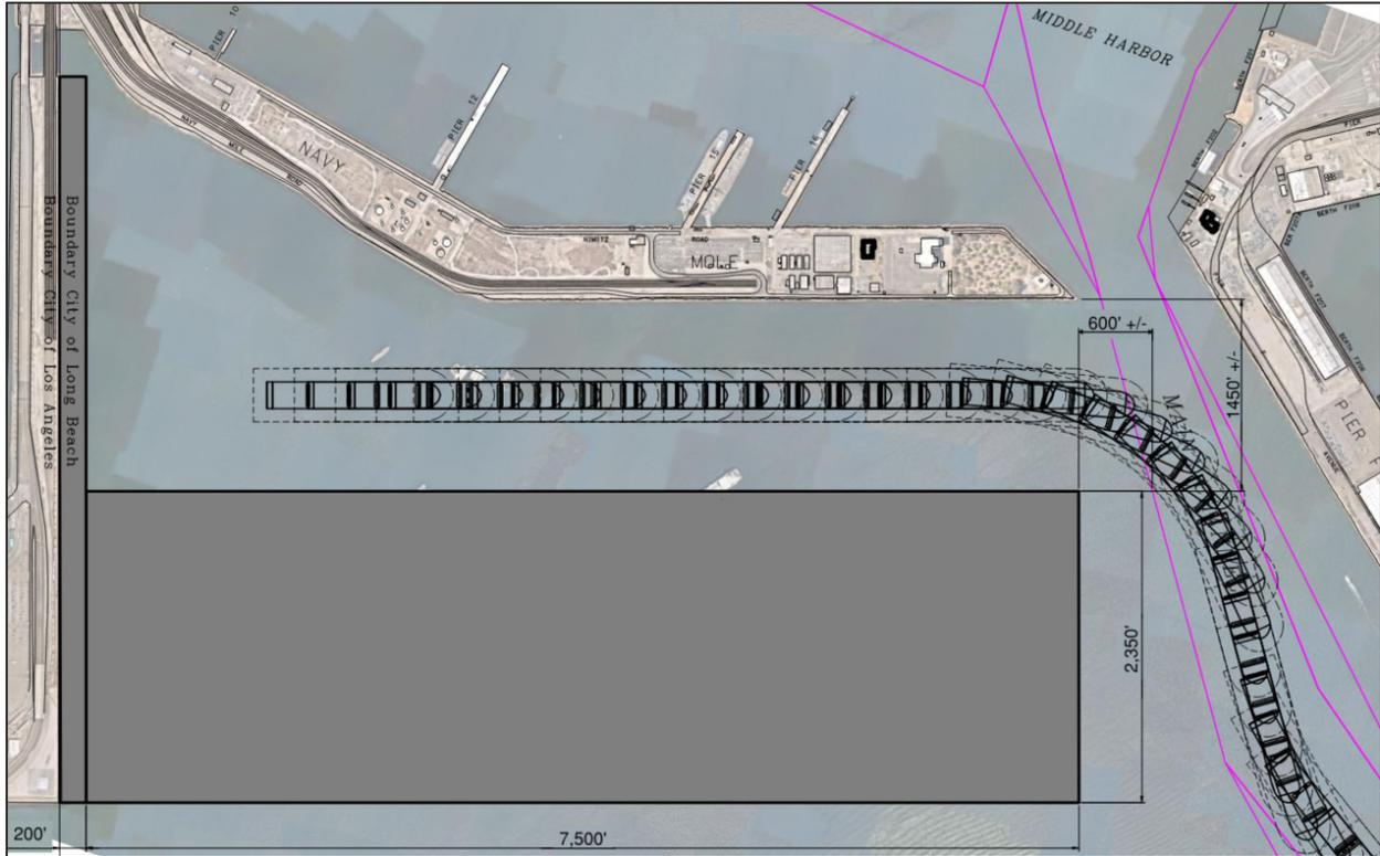
Figure 5: Alternative 1 with Vessel Backing In / Pulling Out
