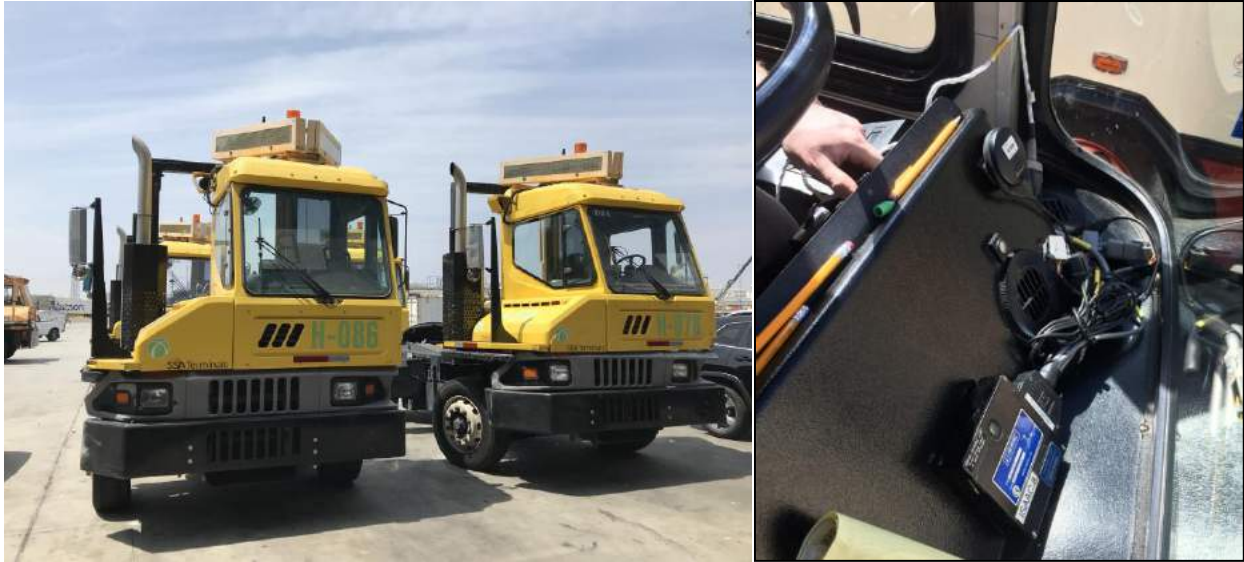
Figure 1.1 Picture of Pier-C yard tractors in POLB (left) and data logger (right)
