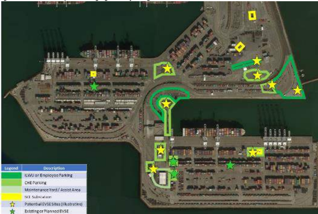
Figure 17: Pier J Conceptual Charging and Refueling Locations
