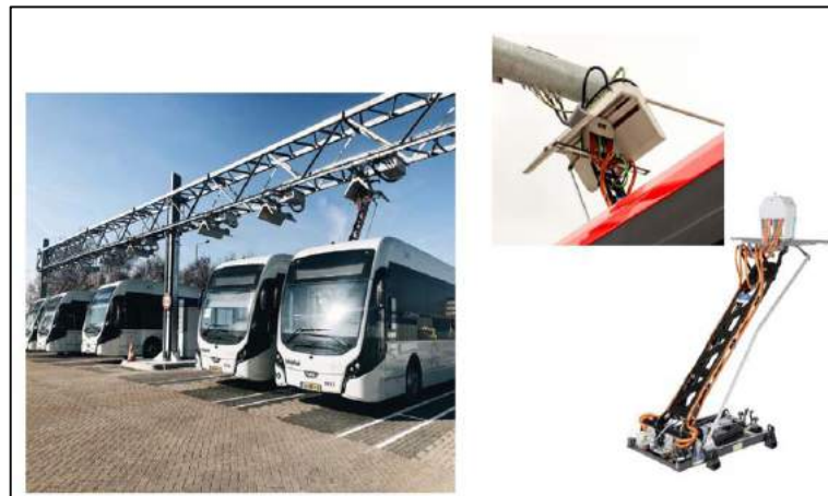
Figure 10. Vehicle-mounted Pantograph Connection (Source: Kosowski 2018)
