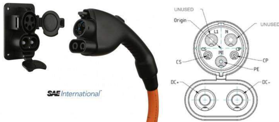
Figure 5. CCS Inlet, Coupler, and Schematic (Sources: Bloomfield 2012, SAE 2017)
