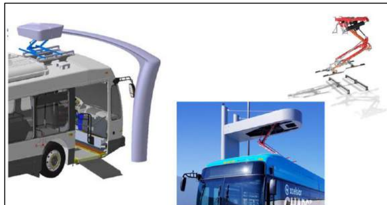
Figure 8. Infrastructure-mounted Cross Rail Connection (Source: Kosowski 2018)
