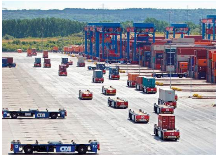
Figure 1: Autonomous container terminal system. AGVs and ASCs pictured. (Dekker & Rotterdam, 2016)
